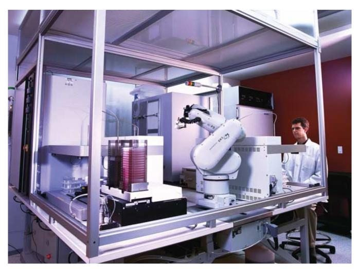
ROBOTIC WORKSTATION in a proteomics facility borrows technology from the assembly lines of the automotive industry. This one is configured to automate repetitive tasks such as pipetting and changing the growth
