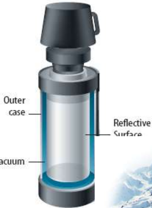
Figure 12 The vacuum layer of the bottle is a very poor conductor of heat.
